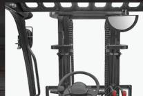
The wide-view mast with optimized design is unlikely to obstruct the operator's line of sight. The enlarged opening size of the fork carriage enables a wider view, a large operation space,
