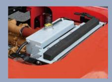
A plate-fin heat dissipater with high-performance fins is used to enable low oil and water temperature without water and oil leakage.
