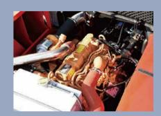
With a high-pressure multiple injection technology, the Bosch-Yuchai high-pressure common-rail engine for the standard configuration has strong output power, less smoke emission, better cold start performance and energy consumption reduced by 109
