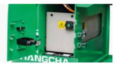
The side movable battery is equipped for standard configuration, which are convenient for battery replacement and repair.
