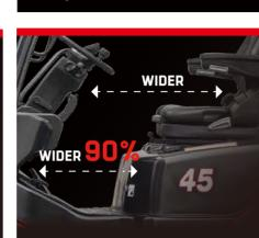
The extra foot space is provided to reduce operator fatigue significantly. The new wide-open, non-slip step makes getting in and out easy and safe.
