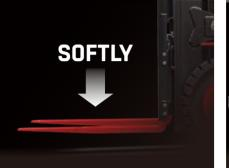
In addition to the soft landing system, the soft lifting system is adopted (front lifting cylinders of triplex mast and full free duplex mast), as a result, the noise and shock of the mast significantly decreases.
