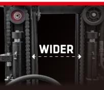
The developed front lifting cylinders with smaller outer diameter give the operator superior forward visibility. The double front lifting cylinders provide better forward visibility.
