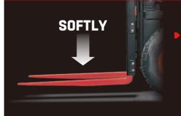
In addition to the soft landing system, the soft lifting system is adopted (front lifting cylinders of triplex mast and full free duplex mast), as a result, the noise and shock of the mast significantly decreases.
