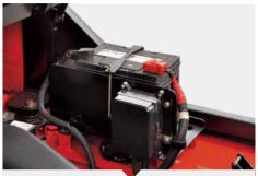
▶ All the controllers, relays, and safety fuses are allocated in the controller box, free to water and dust. The main electronic components are waterproof, which is capable operater in severe environment. And the famous brand air-filter is also applied in the truck.
