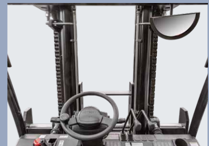
The enhanced mast, frame and steering axle improve the impact resistance of the vehicle
