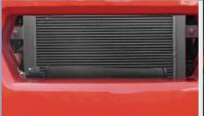
The radiator adopts aluminous plate-fin radiator with better performance and higher structural strength. Impendent oil radiator, optimized oil and water heat dissipation channel and double ventilation holes on counterweight can greatly improve cooling efficiency and reliability of overloaded operation and ensure reliable operation of the engine
